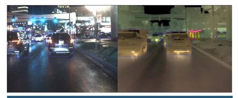
Even in well-lighted areas, thermal images denote pedestrians far more clearly than visible images. Lights from signs and cars do not interfere and the software can distinguish pedestrians from car mufflers.
